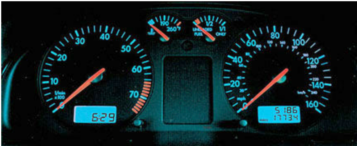
Fig. 3.5. Automotive dashboard back-lit with blue LEDs.
